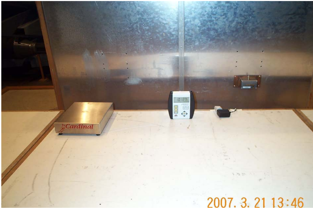
Photo A1.1 Test setup regarding conducted electromagnetic field measurement.
