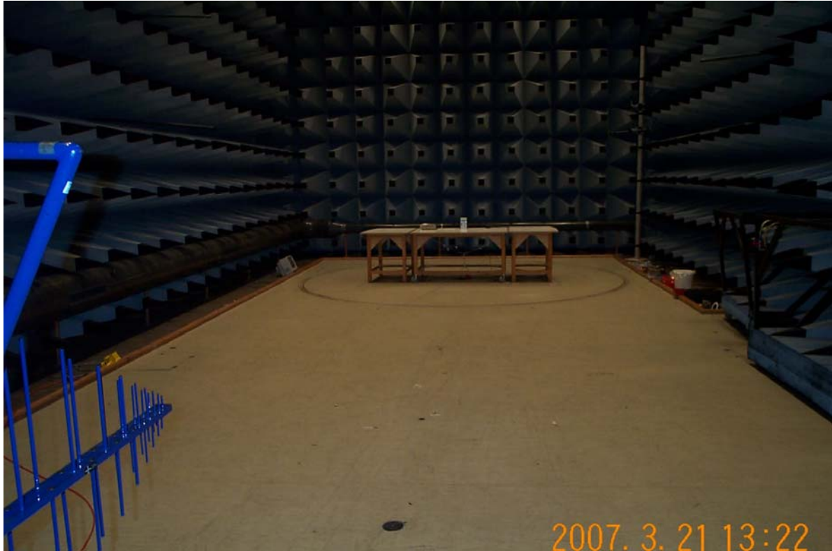
Photo A2.1 Test setup regarding radiated electromagnetic field measurement. Supply: 230 VAC.
