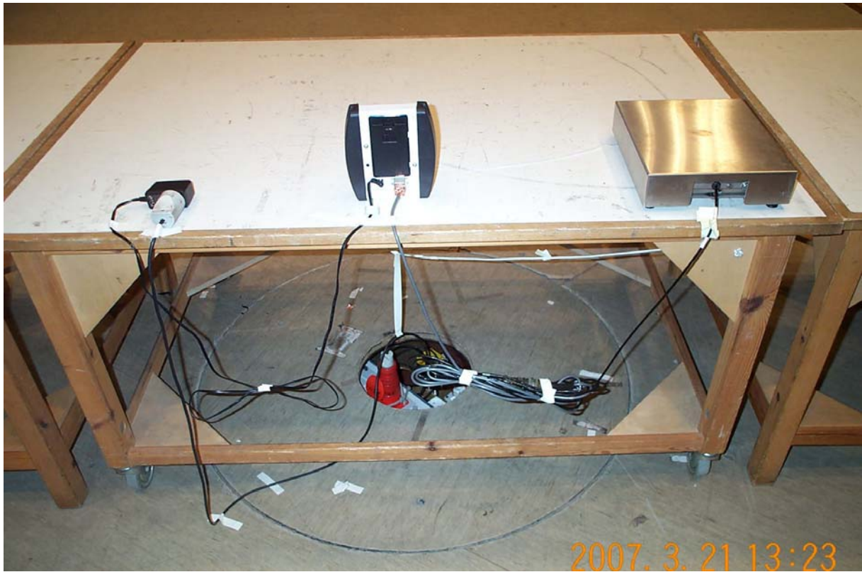
Photo A2.3 Test setup regarding radiated electromagnetic field measurement. Supply: 230 VAC.
